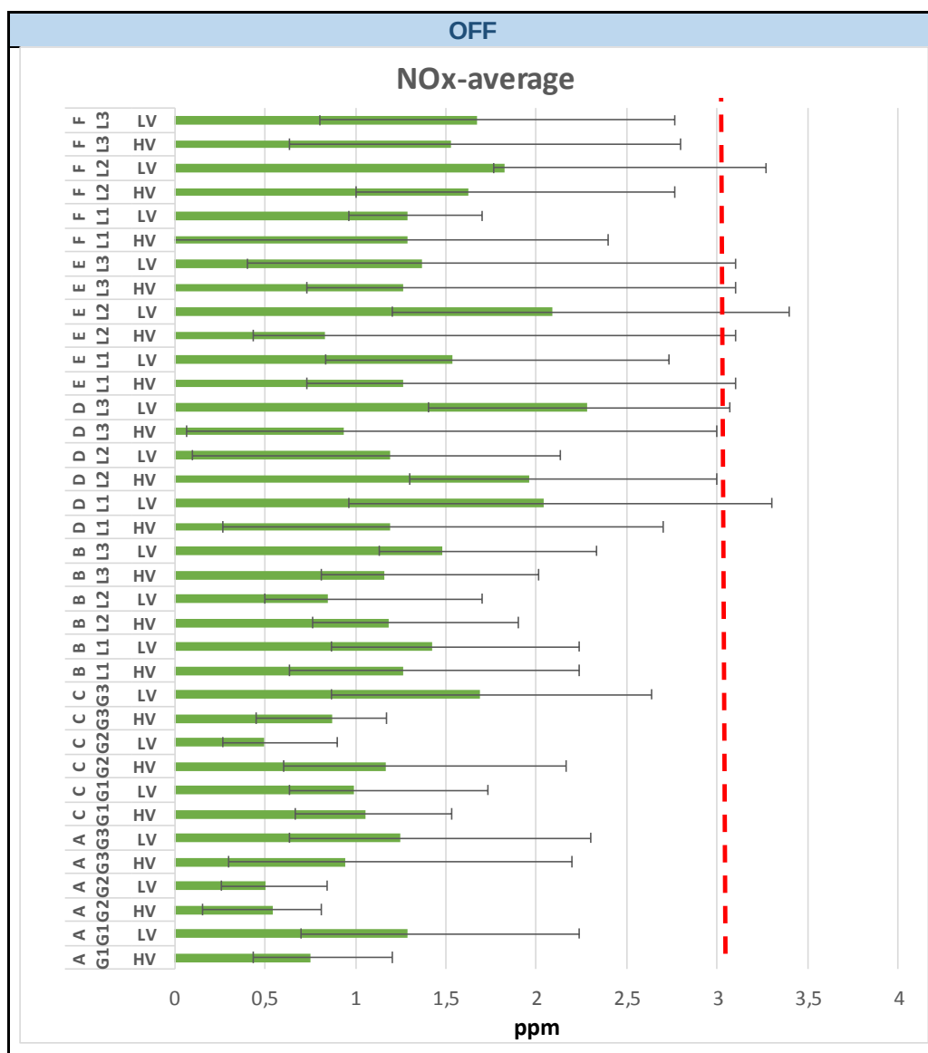
Figure 25 NOx level in ventilated chamber tests in the OFF cycle
