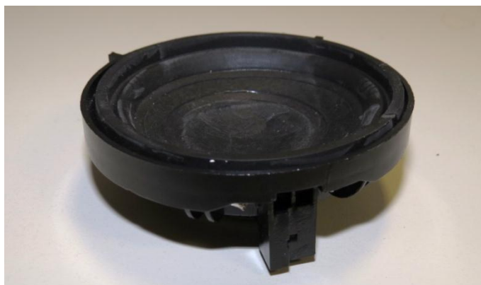
Figure 21: Sample of loudspeaker model B, deliberately damaged by crushing the cone
