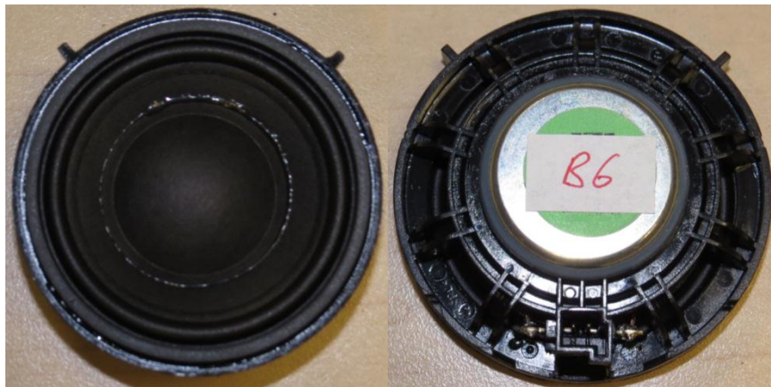
Figure 16: Loudspeaker model B (front and back view), mass: 53 grams, cone diameter: 52 millimetres, in-vehicle location: dashboard
