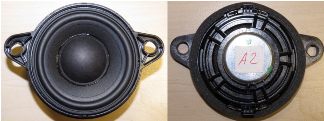
Figure 15: Loudspeaker model A (front and back view), mass: 124 grams, cone diameter: 66 millimetres, in-vehicle location: dashboard
