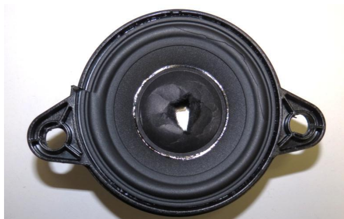
Figure 20: Sample of loudspeaker model A, deliberately damaged by slitting the outer suspension, puncturing the dust cap and cutting open the frame
