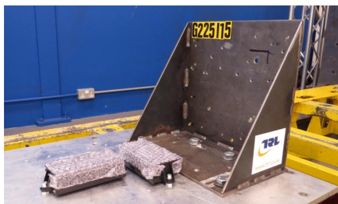
Figure 9: Fujitsu Ten samples mounted on the test sled for horizontal testing
