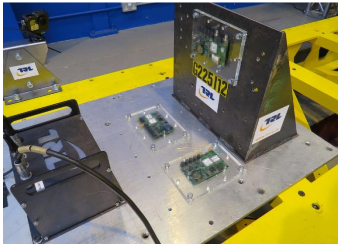
Figure 3: Test setup, detail of horizontal mounting plate and vertical mounting bracket
