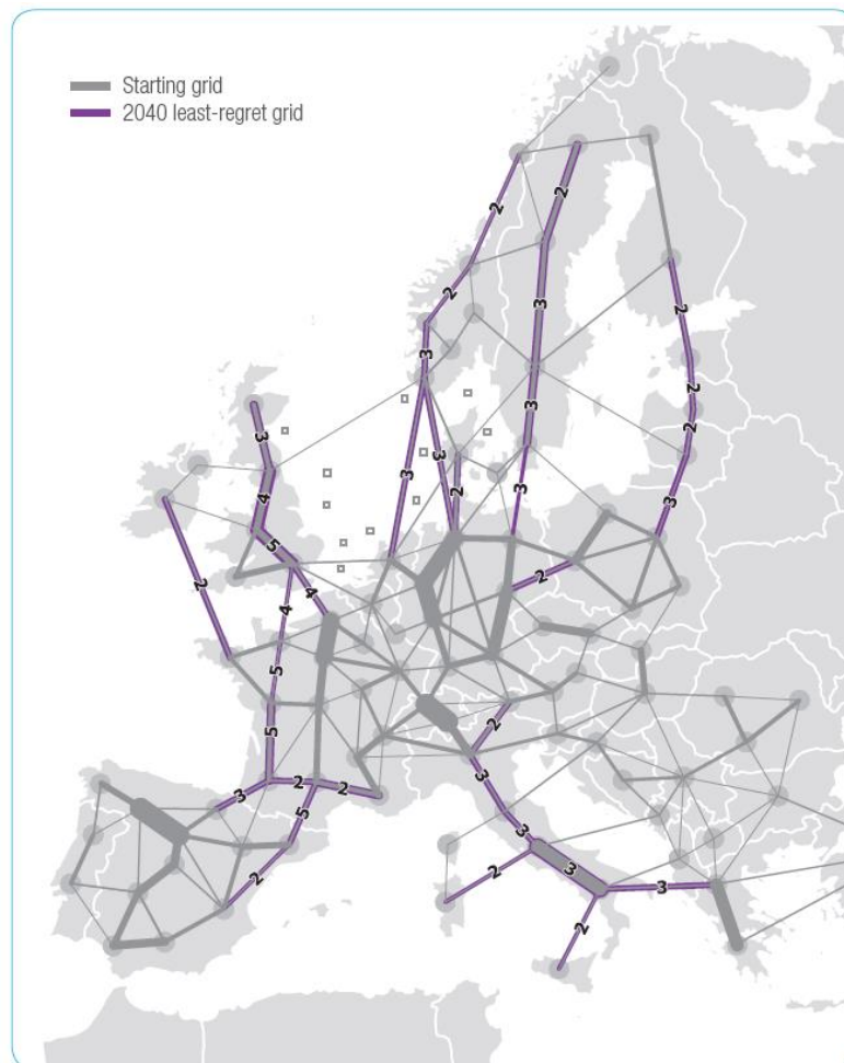
Figure 12. Grid architecture for 2040 covering all scenarios examined (grey: starting grid; purple: reinforcements) as suggested in the 'Electricity Highways 2050' study
